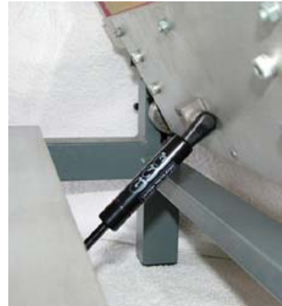
Gas piston stay for easy operation.
